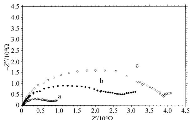
**Fig. 3** Nyquist plots for faradaic impedance measurements of a gold electrode in the presence of 2 mM  $[\text{Fe}(\text{CN})_6]^{3-/4-}$ : (a) bare electrode, (b) Au electrode with self-assembly of a monolayer of ssDNA (probe 2), (c) dsDNA–Au electrode after hybridization with its complementary part.
