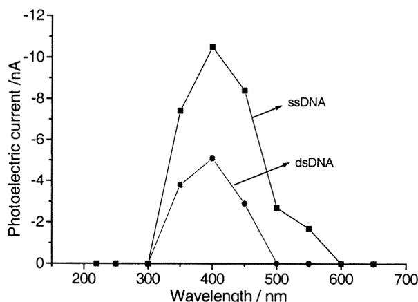
**Fig. 2** The effect of light wavelength on the photocurrent of ssDNA and dsDNA modified electrodes.
