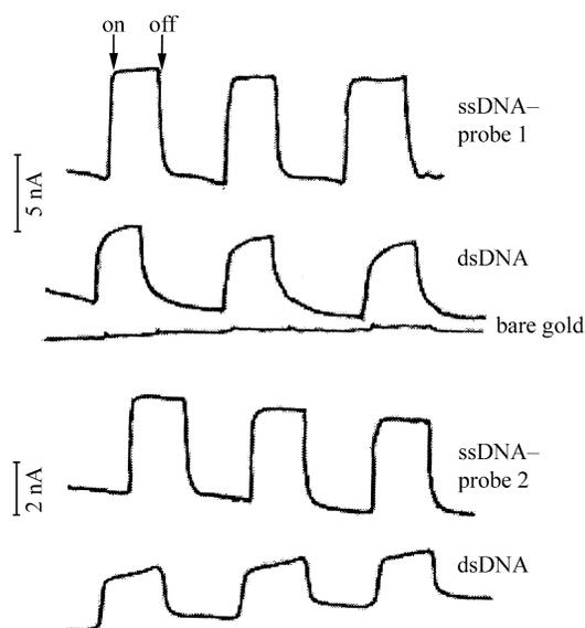
**Fig. 1** Photoelectric behavior of bare gold electrode, ssDNA and dsDNA modified electrodes illuminated with a Xe light power at  $110 \text{ mW cm}^{-2}$  at 200 mV bias voltage.
