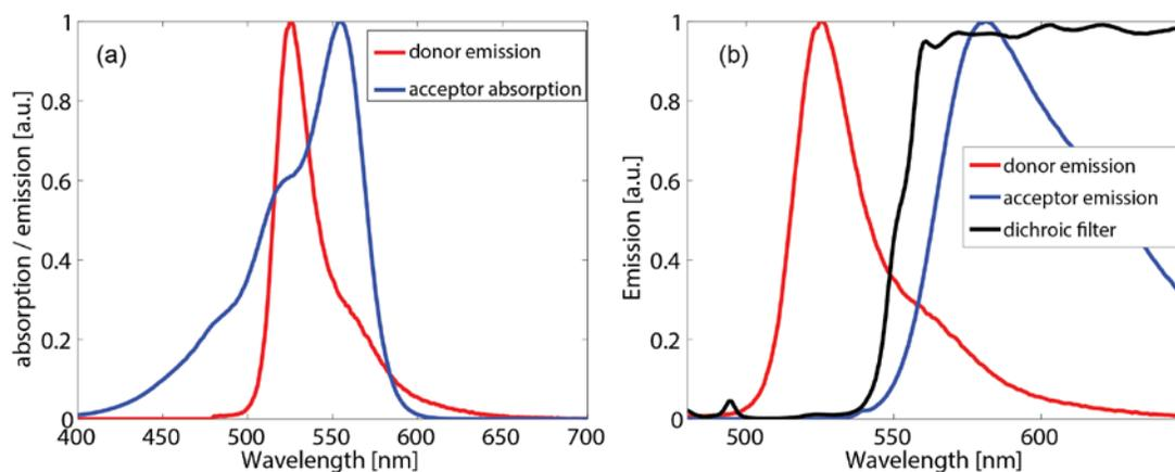
Fig. 1: (a) Overlap of donor (mAmetrine) emission and acceptor (tdTomato) absorption spectrum. (b) Donor and acceptor emission spectra superimposed with transmission profile of the dichroic filter that separates the collected fluorescence into the two detection channels
